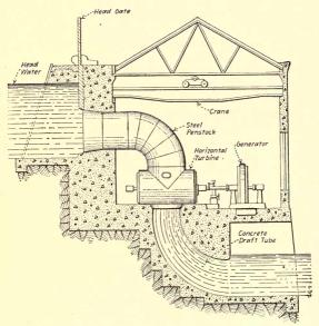
Fig. 294.—A low-head, horizontal-turbo-generator-unit installation. (James Leffel & Co.)
